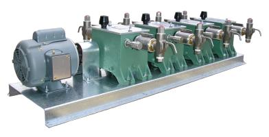
Our 4400 Series is an electric driven injector that can utilize any of the 4 available plunger sizes or three gear ratios with a single head or up to eight heads for a combination of pressure and volume requirements, driven by one motor. The volume pumped can be changed with a simple turn of a micrometer knob from 0-100% of capacity. Also available in corrosion resistant trim.
