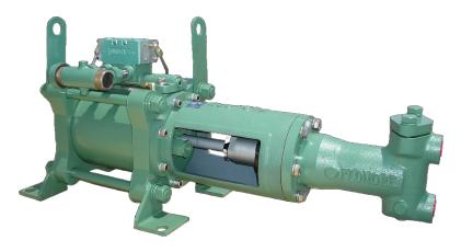
The 6200 series pump consists of a series of basic pump options all developed from a modular power unit. All units are pneumatically driven, positive displacement, single or double acting reciprocation pumps. This pump is used offshore on platforms and onshore at gas plants.
