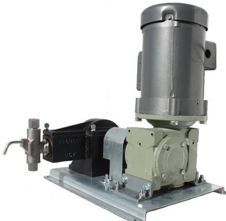
The Flomore 3500 "Wolf" Series pumps are electric driven, positive displacement pumps utilizing C-faced motors and common gear reducers. The 3500 can be configured as a Simplex, Duplex, Triplex, or Quadplex utilizing one gear reducer and motor. The gear reducers are available in 30 and 60 strokes per minute configurations. The 3500 Series can fill many application requirements of different flows and pressures.
